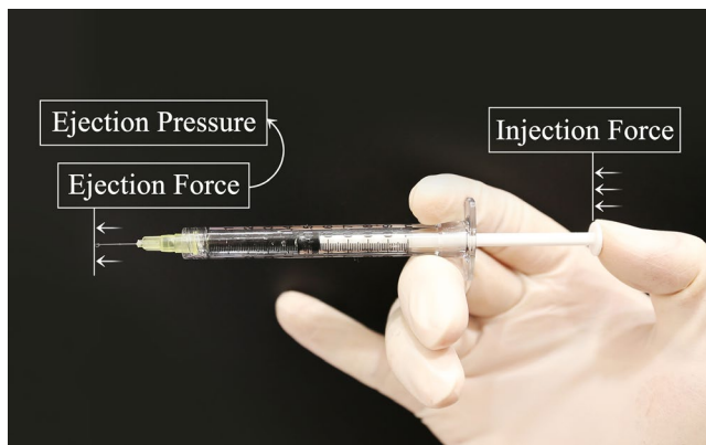
FIGURE 1 Schematic depicting the injection and ejection forces and ejection pressure
